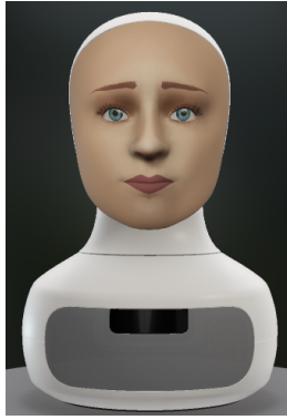
Figure 1: Appearance of the Furhat robot, projecting the ‘Isabel’ face.
